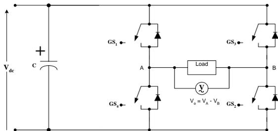
Fig. 1-1. Single-phase inverter
