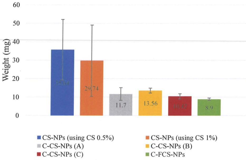
Figure 18: Comparison of particle content in milligram (dried weight of particle in 1 ml) of CS-NPs (using CS 0.5%), CS-NPs (using CS 1%), C-CS-NPs (A), C-CS-NPs (B), C-CS-NPs (C), and C-FCS-NPs.
