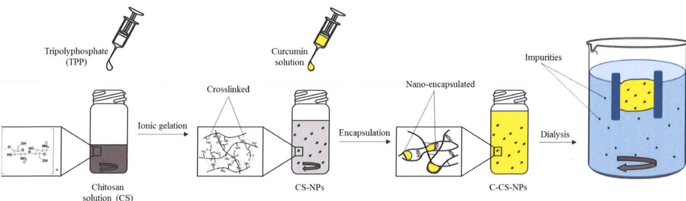
Figure 1: Procedure of encapsulation of curcumin into chitosan nanoparticles (C-CS-NPs)
