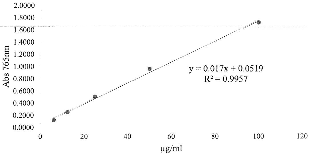
Figure 27: Standard curve of gallic acid for evaluation of total phenolic content
