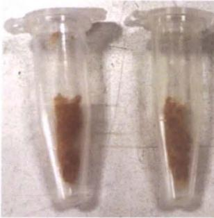
Figure 15: Freeze dried curcumin and folate-conjugated chitosan nanoparticles (C-FCS-NPs)
