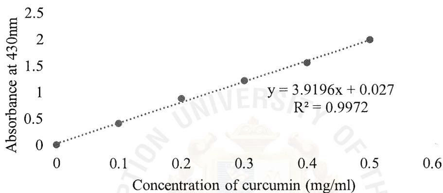
Figure 26: Standard curve plotted between absorbance at 430nm and concentration of curcumin (mg/ml)
