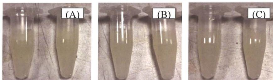
Figure 5: Curcumin encapsulated-chitosan nanoparticles (C-CS-NPs) using A (adding curcumin after nanoparticle formation), B (adding curcumin before nanoparticle formation by mixing curcumin with TPP), C (adding curcumin before nanoparticle formation by mixing curcumin with CS).
