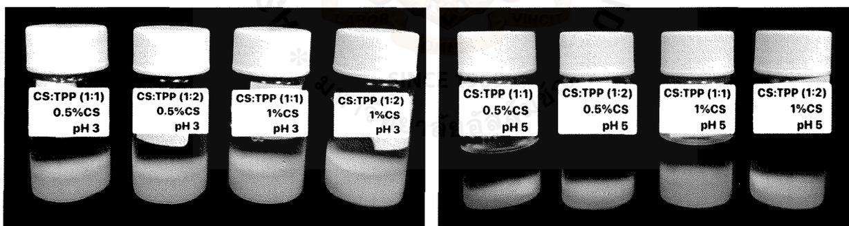
*Figure 3: Formulation of CS-NPs at concentrations of 0.5%CS and 1%CS, different ratio of CS to TPP at pH 3 and pH 5*
