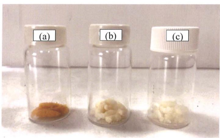
Figure 19: Freeze dried form of C-FCS-NPs (a), C-CS-NPs (b) and CS-NPs (c) using 0.5%CS, and method C for encapsulation of curcumin
