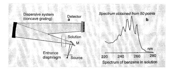
Figure 2.9. Multichannel Detection.
