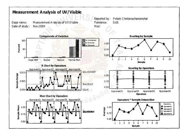
Figure 4.1. Gage R&R Graphical Output.
