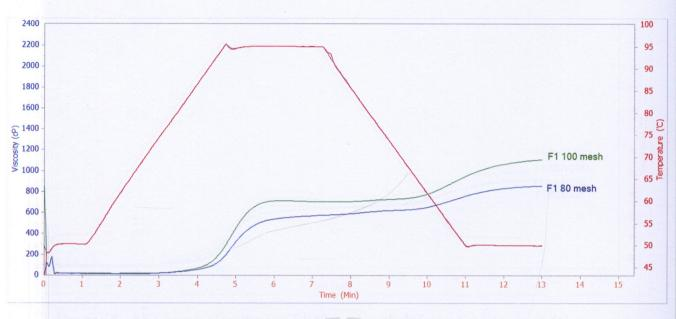
Figure 12: RVA graph of 100 mesh and 80 mesh particle size of flour
