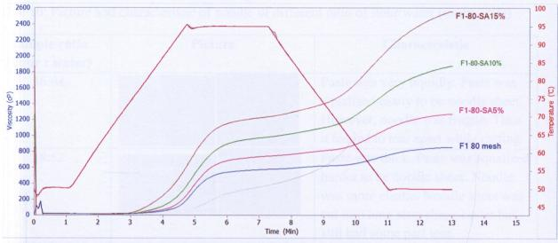
1. Figure 16: RVA graph of mixture of F1 80 mesh with different percentage of SA
