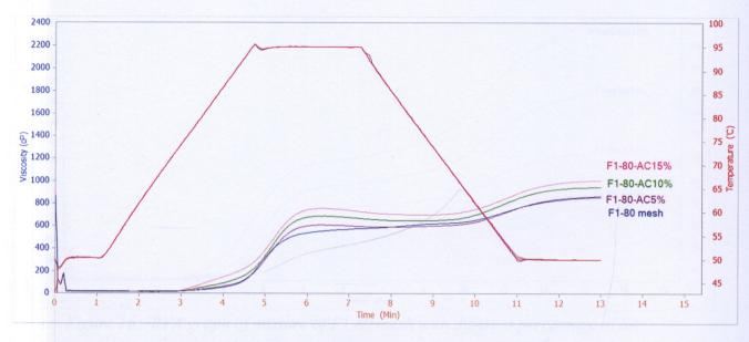
1. Figure 14: RVA graph of mixture of F1 80 mesh with different percentage of AC
