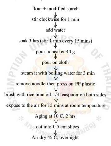
Figure6: Modified starch added noodle production
