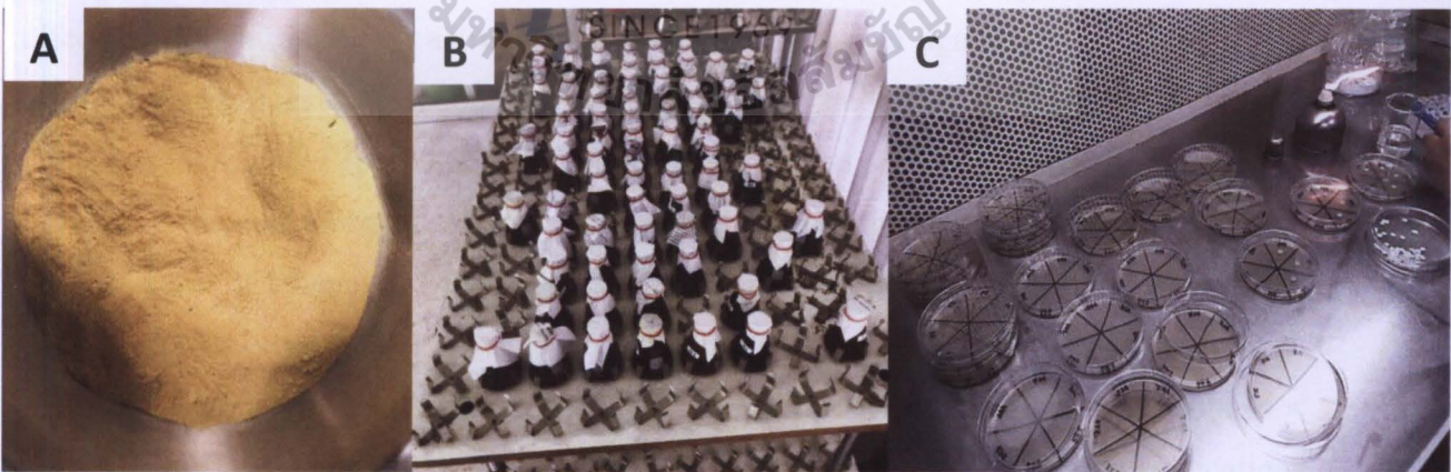
Figure 7: Experimental procedure: A - Powdered raw material, B- extraction process and C - laboratory testing of antimicrobial activity
