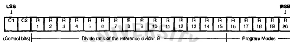
Figure A.1 R Counter for RF and IF
