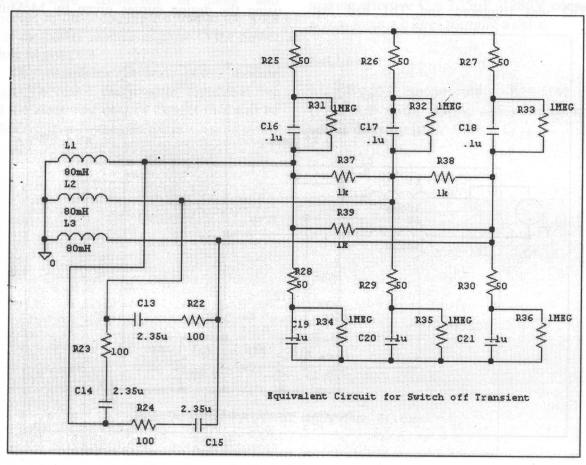
=  $50\Omega$  - 50W, C =  $2.35\mu F$  - 1280V. The surge suppressor was connected between lines and forms a delta connection. For those who are interested in the pspice simulation, the circuit used for this purpose is given below with the condition that the R-phase magnetizing current is maximum at the time of transformer disconnection.
